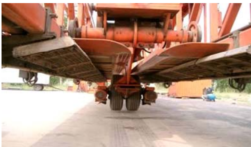
图 2-22 加速加载试验系统(Accelerated Loading Facility)
