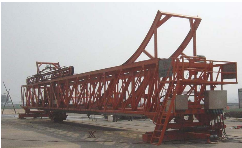
图 2-21 加速加载试验系统(Accelerated Loading Facility)
